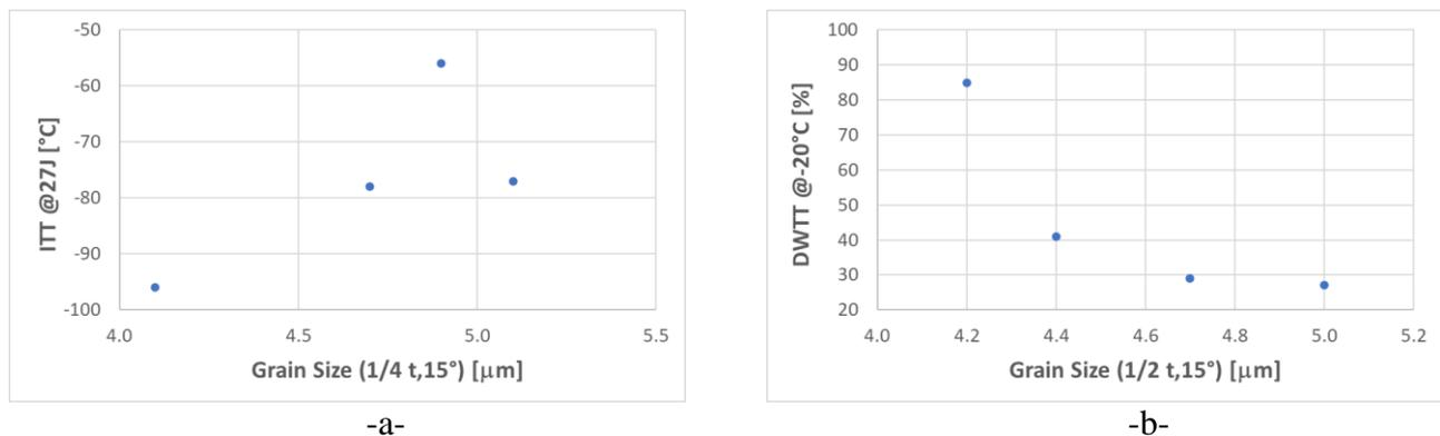
Figure 4: Correlation between grain size and (a) impact transition temperature at 27 J measured by Charpy tests and (b) ductile fraction in fracture area measured by DWTT observed in the strips studied in this work.
