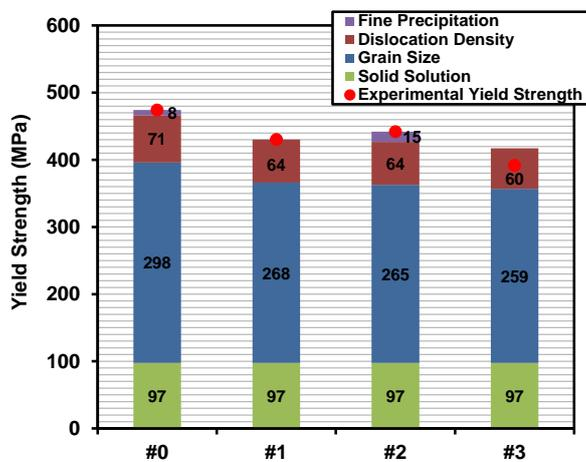
Figure 3: Calculated contributions of several strengthening mechanisms to the yield strength of the strips studied in this work.
