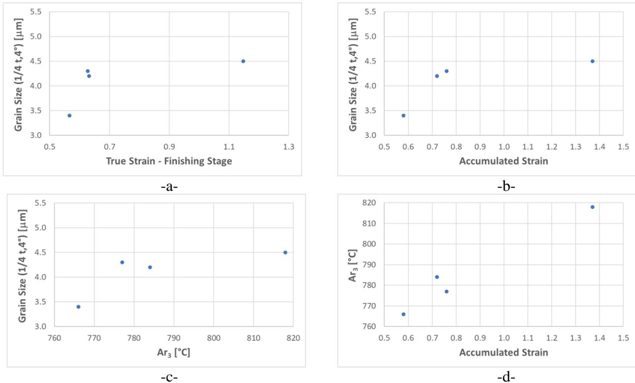
Figure 5: Measured mean ferritic grain size at 1/4 thickness in function of the evolution of (a) true strain in the TMCP finishing stage, (b) accumulated strain of austenite immediately after TMCP, calculated by the MicroSim model, and (c)  $A_{r3}$  temperature as calculated by the PhasTransSim model.  $A_{r3}$  temperatures in function of accumulated strain at rolling end as calculated by MicroSim are shown in (d).
