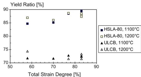
Fig. 4. Evolution of the yield ratio of the HSLA-80 (aged) and ULCB (as rolled) steels according to the total strain applied during the rolling tests.
