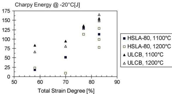
Fig. 6. Evolution of the Charpy energy absorbed at  $-20^{\circ}\text{C}$  of the HSLA-80 (aged) and ULCB (as rolled) steels according to the total strain applied during the rolling tests.
