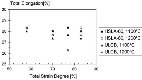
Fig. 5. Evolution of the total elongation of the HSLA-80 (aged) and ULCB (as rolled) steels according to the total strain applied during the rolling tests.
