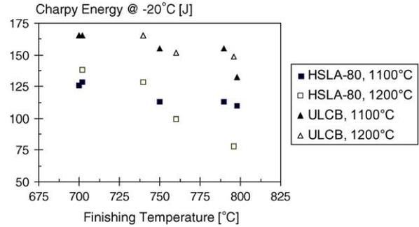
Fig. 11. Evolution of the Charpy energy absorbed at  $-20^{\circ}\text{C}$  of the HSLA-80 (aged) and ULCB (as rolled) steels according to the finishing temperature applied during the rolling tests.
