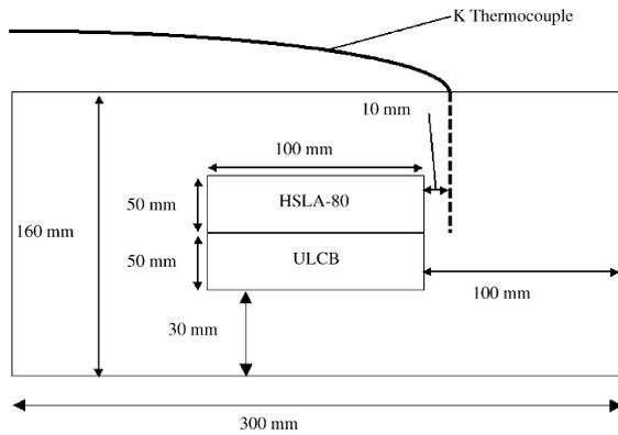
Fig. 1. Hot rolling set composed of the HSLA-80 and ULCB steel blocks for hot rolling embedded in a welded steel frame. This device allowed the simultaneous hot rolling of a sample of each steel, assuring that they were subjected exactly to the same parameters of the thermomechanical treatments.
