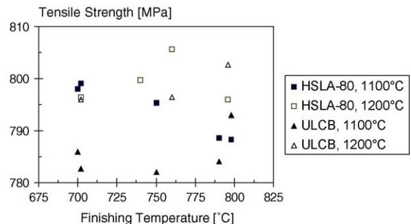
Fig. 8. Evolution of the tensile strength of the HSLA-80 (aged) and ULCB (as rolled) steels according to the finishing temperature applied during the rolling tests.
