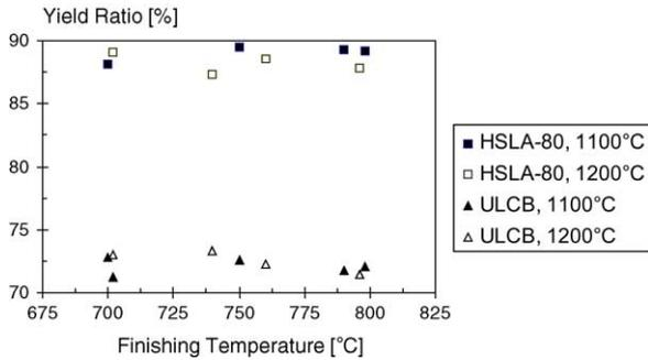
Fig. 9. Evolution of the yield ratio of the HSLA-80 (aged) and ULCB (as rolled) steels according to the finishing temperature applied during the rolling tests.
