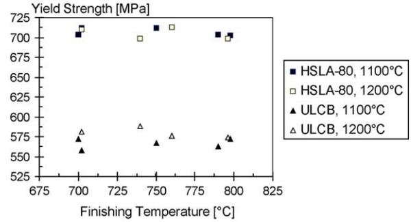
Fig. 7. Evolution of the yield strength of the HSLA-80 (aged) and ULCB (as rolled) steels according to the finishing temperature applied during the rolling tests.
