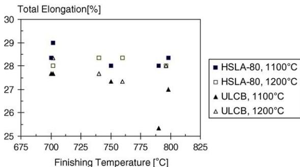
Fig. 10. Evolution of the total elongation of the HSLA-80 (aged) and ULCB (as rolled) steels according to the finishing temperature applied during the rolling tests.
