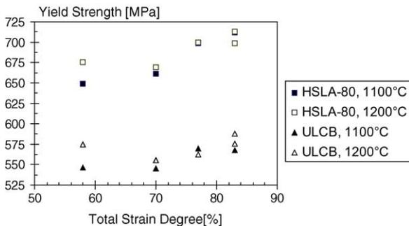
Fig. 2. Evolution of the yield strength of the HSLA-80 (aged) and ULCB (as rolled) steels according to the total strain applied during the rolling tests.
