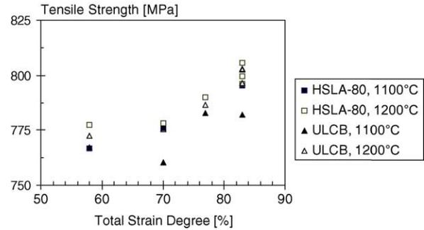
Fig. 3. Evolution of the tensile strength of the HSLA-80 (aged) and ULCB (as rolled) steels according to the total strain applied during the rolling tests.
