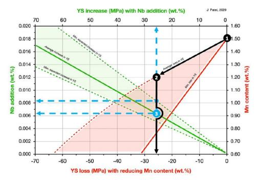
**Figure 2:** Abacus to determine the addition of niobium that is necessary to compensate for the loss of yield strength resulting from the reduction of the manganese content in structural steels with yield strength less than or equal to 355 MPa [7].
