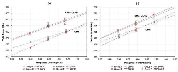
**Figure 4:** Effect of manganese content on (a) yield stress and (b) tensile stress) for CMn (Group A) and ULNb (Group B) steels, considering finish rolling temperatures of 950°C and 900°C [1].
