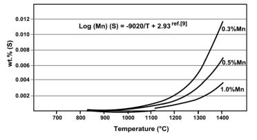
Figure 8: Sulphur solubility curves in austenite as a function of temperature and Mn content [12].
