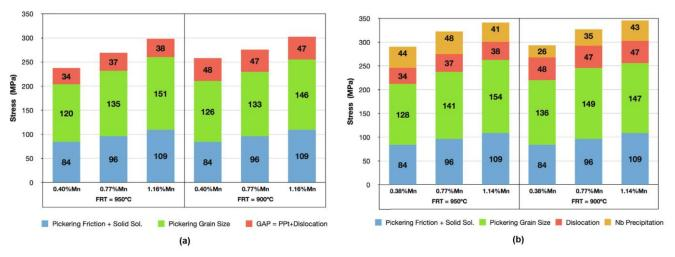
**Figure 7:** Breakdown of individual strengthening components for (a) Group A and (b) Group B steels [1].
