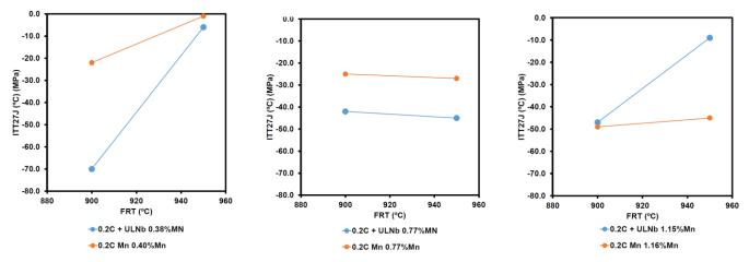
Figure 6: Effect of finish rolling temperature on impact transition temperature at 27 J for CMn (Group A) and ULNb (Group B) steels [11].
