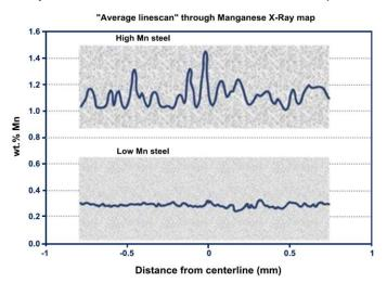
Figure 9: Segregation intensities for steels with high (top chart) and low (bottom chart) manganese contents [12].
