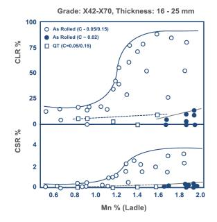
Figure 10: Effect of manganese content in steel on its susceptibility to hydrogen cracking, expressed in terms of crack length ratio (top graph) and crack sensitivity ratio (bottom graph) [12].
