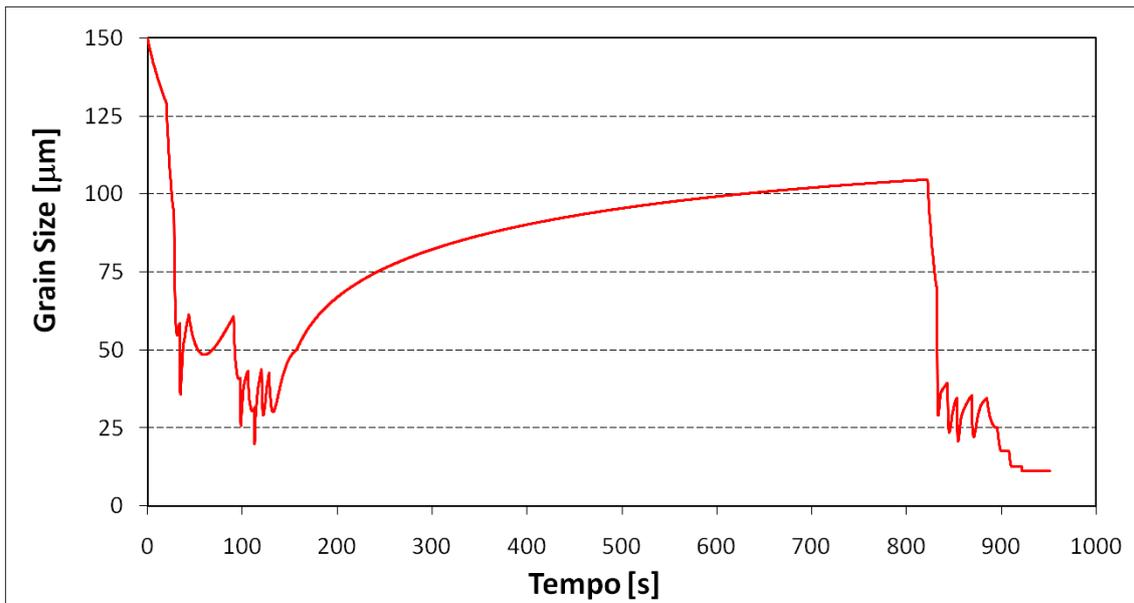
Figure 6: Grain size evolution predicted during normalizing rolling of a 0.15%C, 0.020% Nb and 0.0085% N steel according to the default pass schedule described here.
