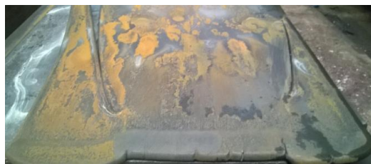
Figure 8. Example of slab thermal expansion corner cracking of 690 Mpa yield strength titanium precipitation strengthening grades. Slab corner after reheating, rolled slab after roughing.
