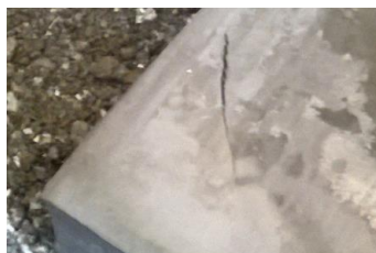
Figure 8. Example of slab thermal expansion corner cracking of 690 Mpa yield strength titanium precipitation strengthening grades. Slab corner after reheating, rolled slab after roughing.
